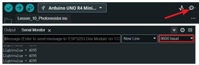
The detection value is <300 when covering the photoresistor with objects.
