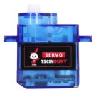
The steering gear (servo motor) control pulse signal period is a 20MS pulse width modulation signal (PWM), the pulse width is from 0.5ms to 2.5ms, and the corresponding steering position changes linearly from 0 to 180 degrees.
