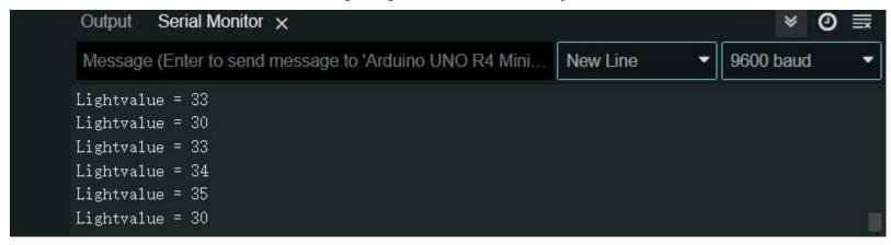
When the photoresistor is illuminated with a flashlight, the detection value is >1000.
