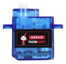
The steering gear (servo motor) control pulse signal period is a 20MS pulse width modulation signal (PWM), the pulse width is from 0.5ms to 2.5ms, and the corresponding steering position changes linearly from 0 to 180 degrees.
